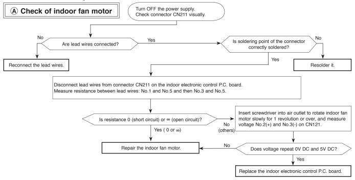
Indoor unit operates by pressing the EMERGENCY OPERATION switch, but doesn't operate with the remote controller.
